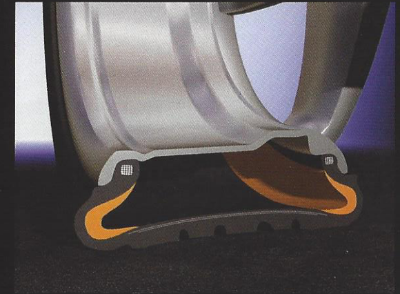
Reinforced so you can continue to drive if it loses air pressure
